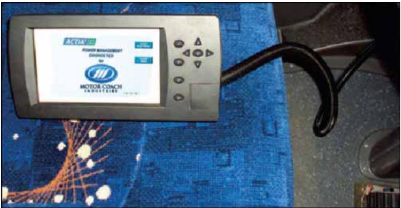
**Figure 49. LCD diagnostic interface connected underneath the instrument panel.**
