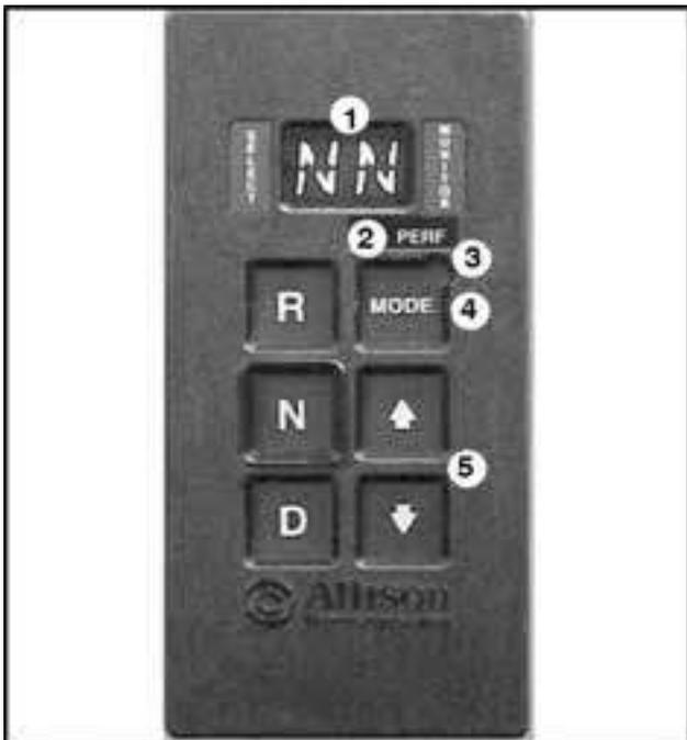
Figure 54. GEN V pushbutton shift selector
